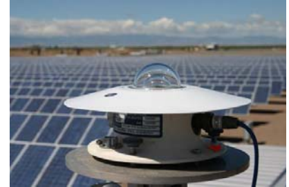
A pyrheliometer at the SunEdison photovoltaic (PV) power plant measures solar radiation from the sky dome. Photo Courtesy NREL.
