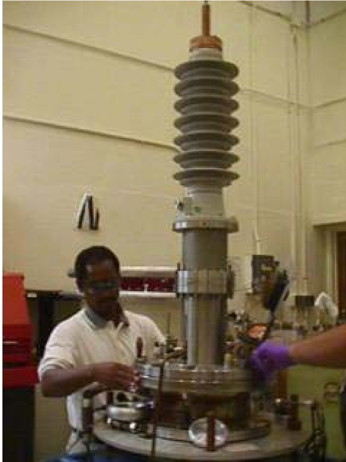
Testing Cryogenic Performance of Bushing Insulating Materials at ORNL
