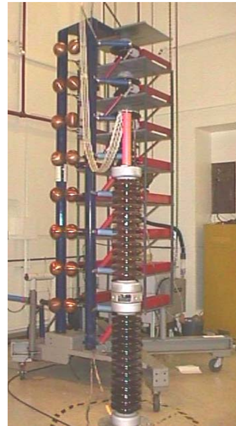
800 kV lightning impulse generator
